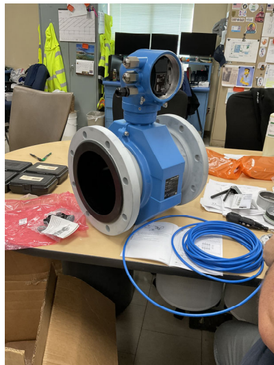
Staff bench testing new flowmeter (left) and new flowmeter installed at Weymouth plant (right).
