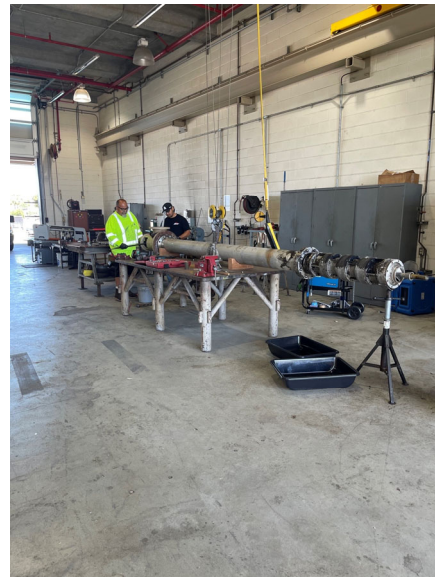
Staff rebuilding a vertical turbine pump at the Diemer plant.
