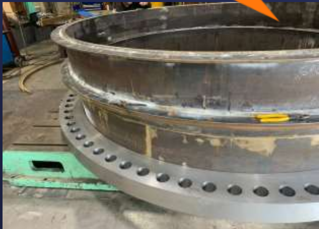
New Slip Joint Fabrication @ La Verne Shops
