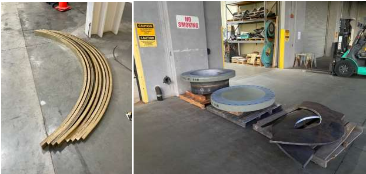
Rolled compression ring segments (left) and fabricated 36-inch spool assembly (right) for Upper Feeder repairs
