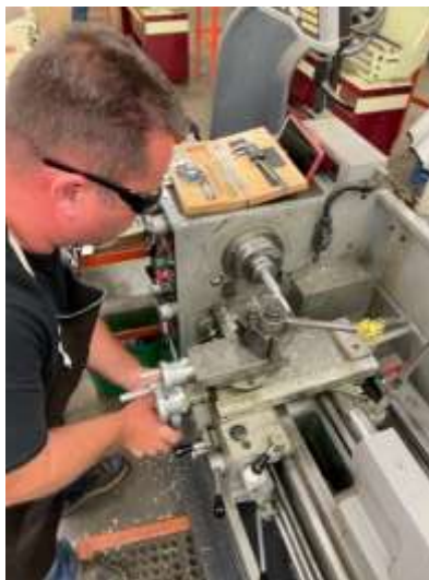
Apprentice using a lathe to machine a taper
