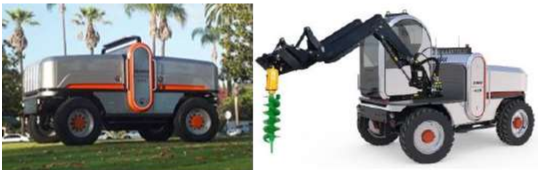
Examples of the all-electric mobile power station basic version (left) and backhoe version with drill attachment (right)
