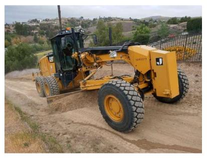
Staff using a motor grader for patrol road repairs along the Lower Feeder
