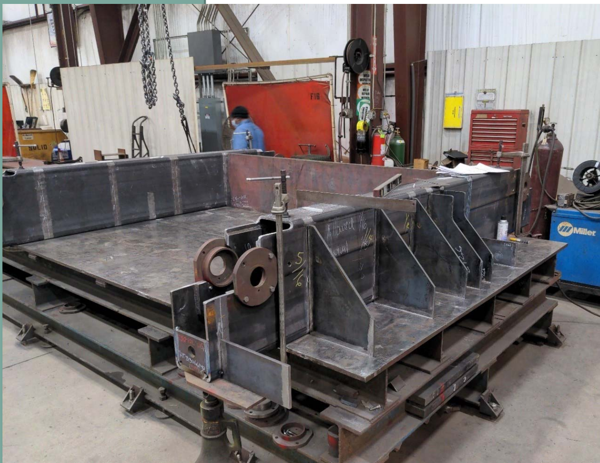
Fabrication of hoist for new CRA Pumping Plant overhead crane
