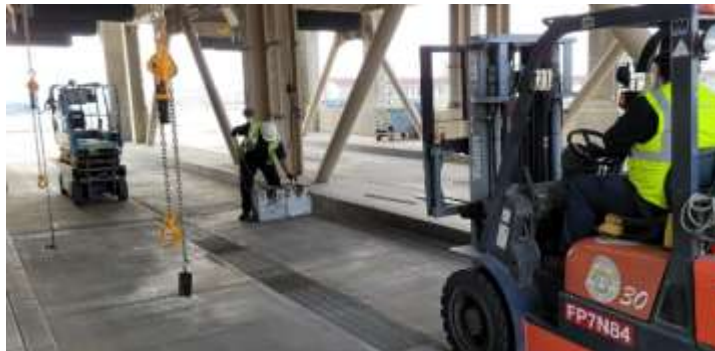
Staff preparing to suspend weights from the solids hopper at the Weymouth plant
