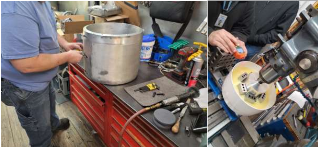
Staff performing measurements of the bearing seal (left) and evaluating performance of improvements on a scale model (right) at Yorba Linda HEP
