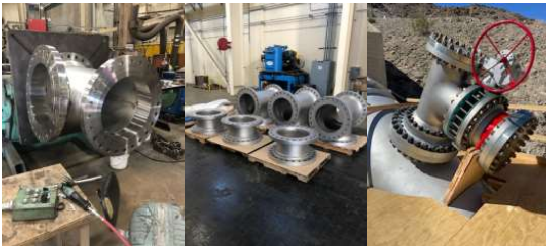
Fabrication of re-circulation line components (left and center) and installed tee (right) for Eagle Mountain pumping plant
