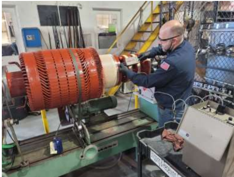
Staff overseeing final electrical testing of a pump unit's armature for Hinds pumping plant
