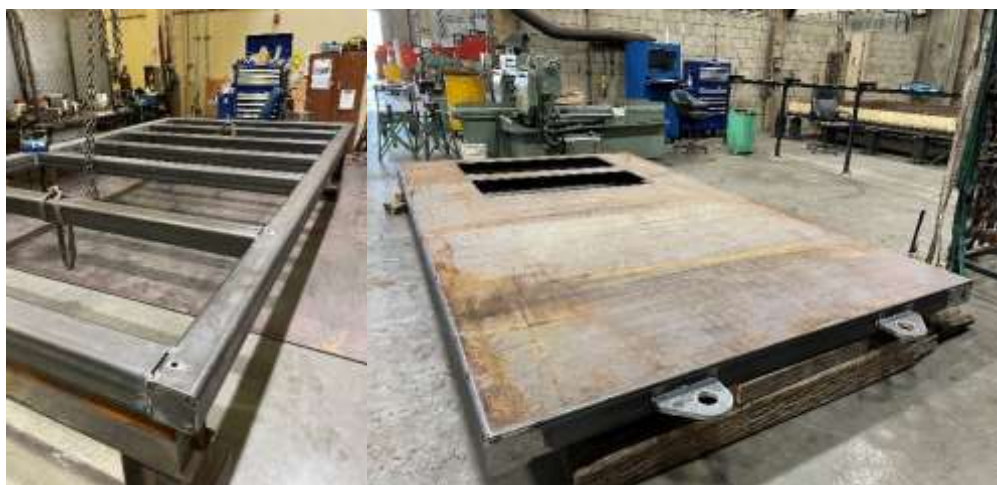
Fabrication of gate frame (left) and installed gate skin with square openings (right) for Desert pumping plants
