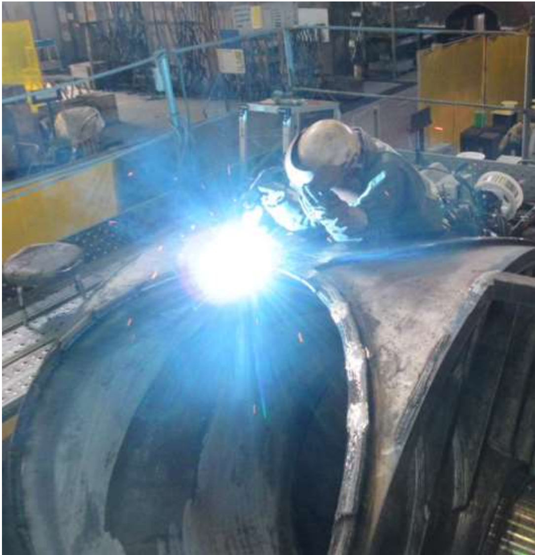
Second Lower Feeder Isolation Valve Procurement—Welding on the 54-Inch Diameter Conical Plug Valve
