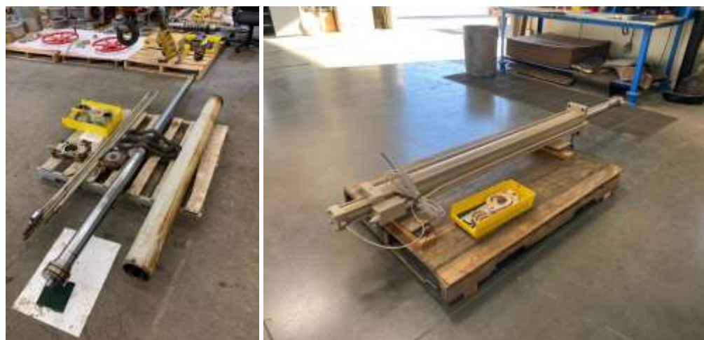
Disassembly of hydraulic rams at the La Verne Shops
