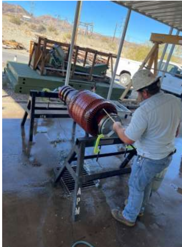
Staff cleaning a synchronous motor armature used for CRA pumps
