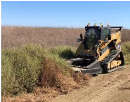
Staff using a skid steer with brush mower attachment to remove brush along the Lower Feeder
