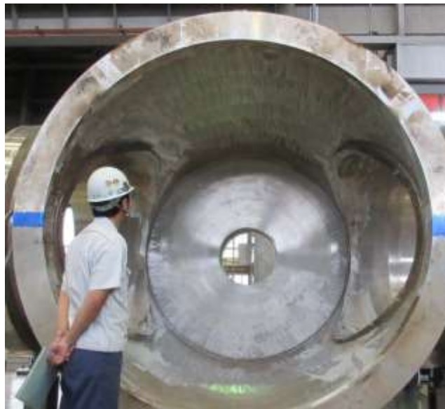
Second Lower Feeder Isolation Valve Procurement —Fabrication of 54-inch diameter valve body
