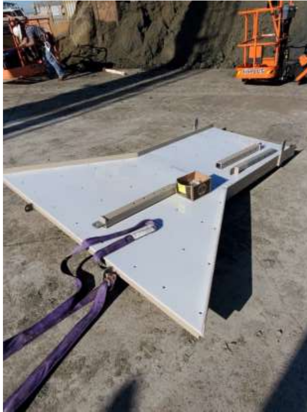
Newly fabricated conveyor chute prepared for installation at the Skinner plant
