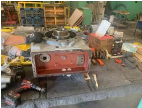
Reassembly of the valve actuator before (left) and after (right) testing and coating work at the La Verne Shops
