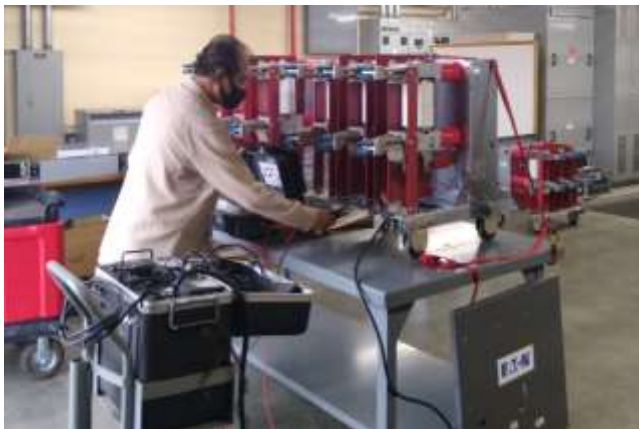
Staff performing high-voltage testing on vacuum-style circuit breakers (left) and electrical testing on instrument transformers (right) at the Weymouth plant
