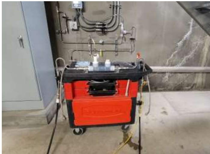
Ozone calibration cart with standby analyzer and probe at the Weymouth plant
