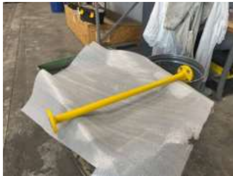
Fabricated spool assembly for the ammonia feed system at the Jensen plant
