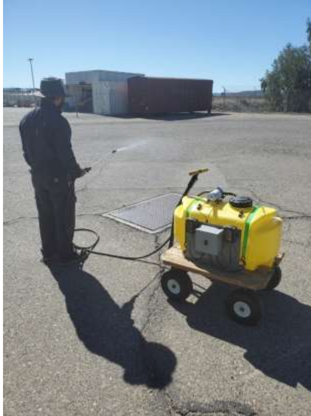
Portable battery-powered disinfection sprayer invented at the Skinner plant
