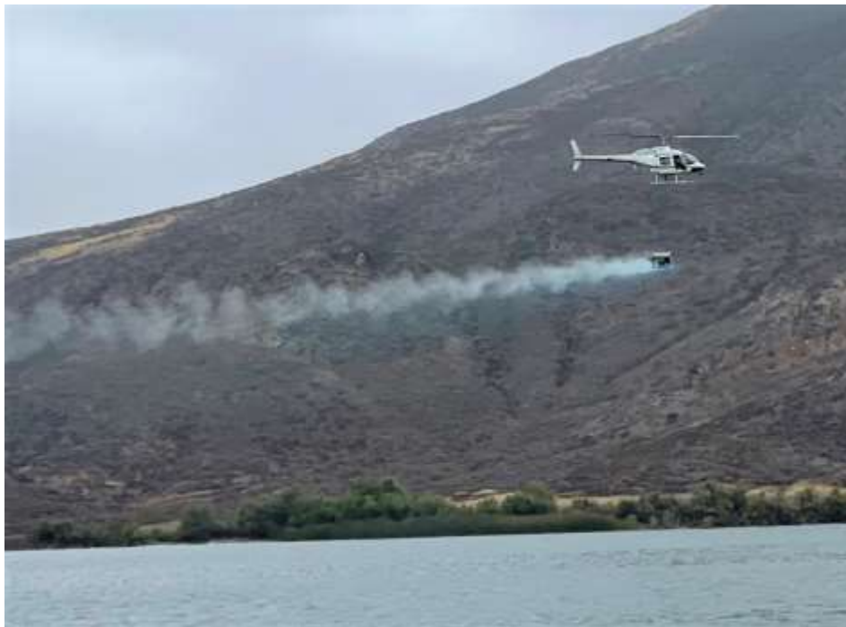
Treating Lake Skinner with copper sulfate to control a problematic cyanobacterial bloom
