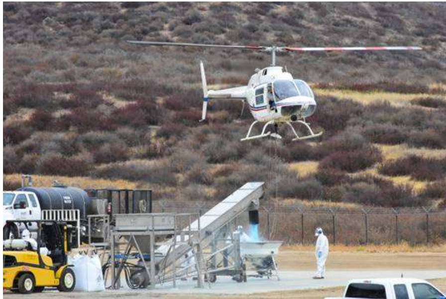
Staff loading copper sulfate in the spreader bucket at Lake Skinner
