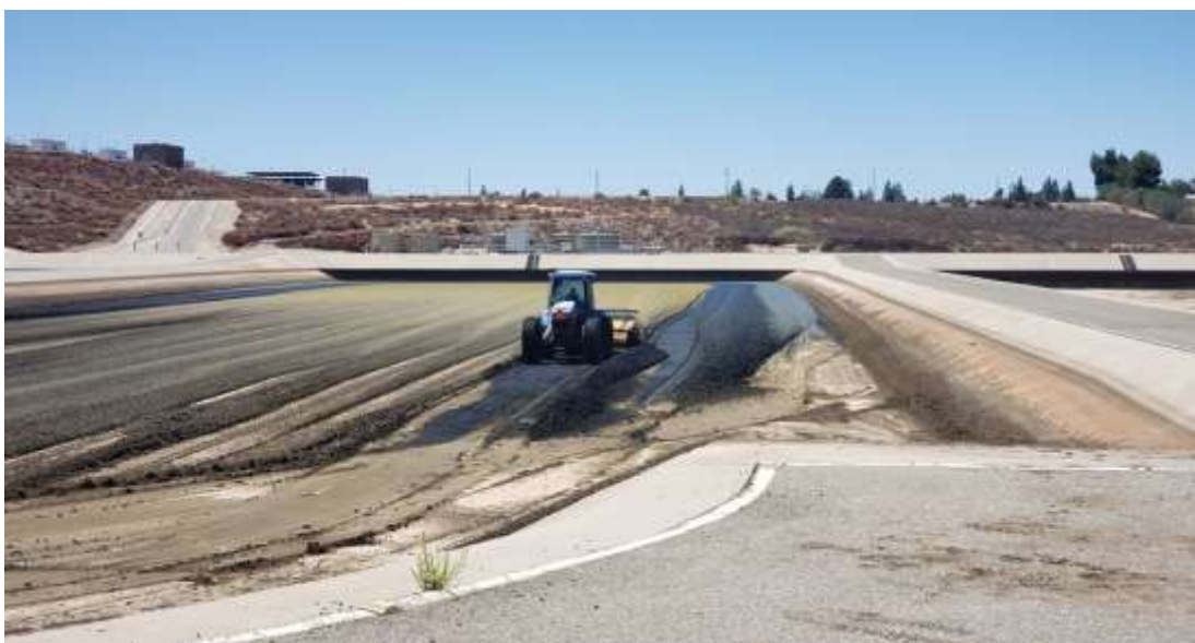
Brown Bear moving wet solids in to windrows to aid in drying at the Mills plant
