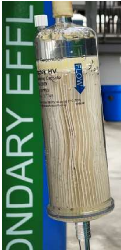
Secondary effluent samples are concentrated onto a 1-micron filter for pathogen analysis at the demonstration facility
