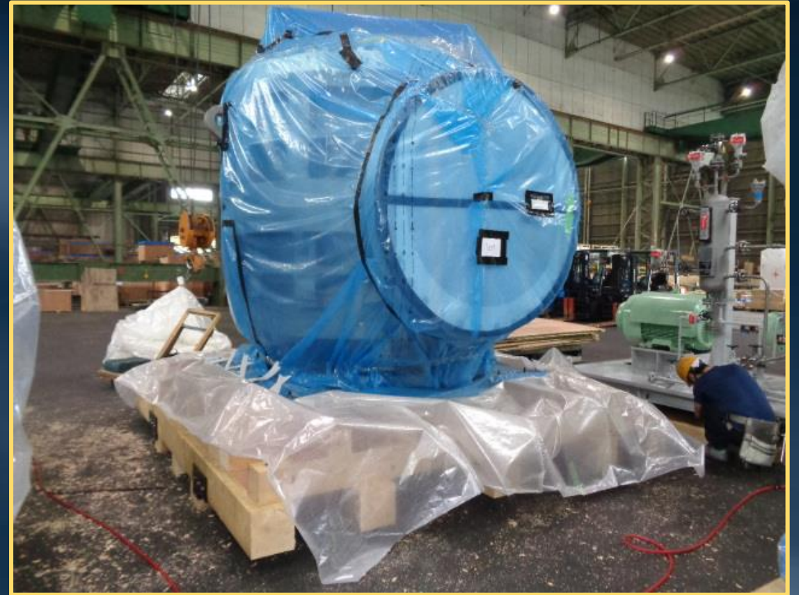
48-inch valve fabrication and packaging prior to shipment
