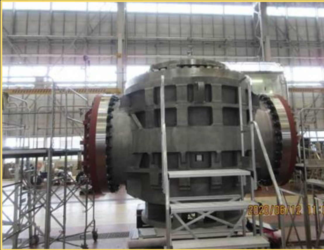
48-inch valve fabrication and packaging prior to shipment
