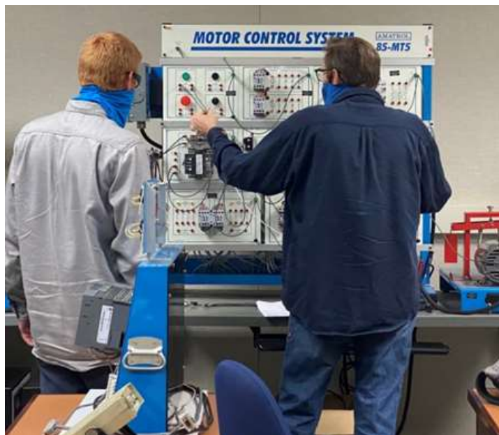
Class of 2023 apprentice and subject matter expert reviewing wiring specifications on motor control simulator
