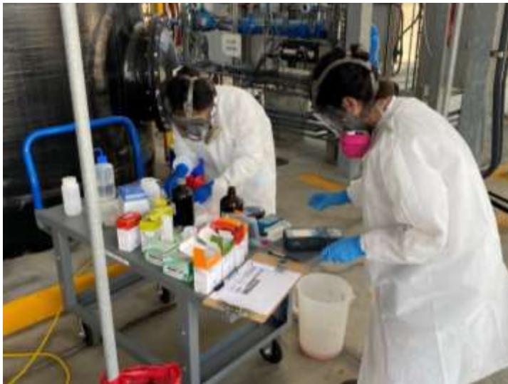
Consultant staff perform 1,4-dioxane challenge testing on the advanced oxidation process at the demonstration facility
