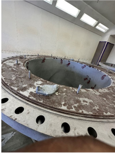
Corrosion on top side (left) and finished coating (middle and right) of a component of the DVL sleeve valve
