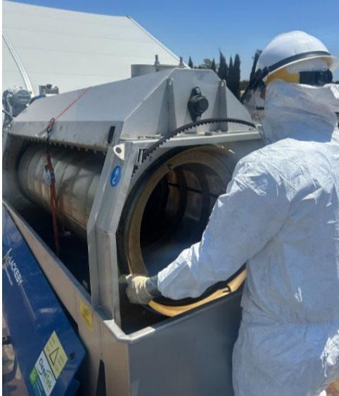
Maintenance on drum screening equipment (left) and newly installed hazardous waste accumulation area (right) at the Napolitano Innovation Center
