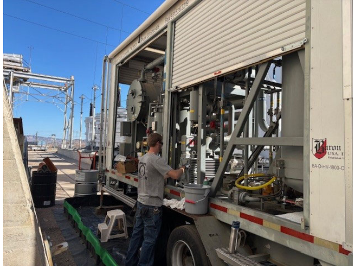
Staff operating a mobile oil purification unit to maintain transformers at the Gene pumping plant
