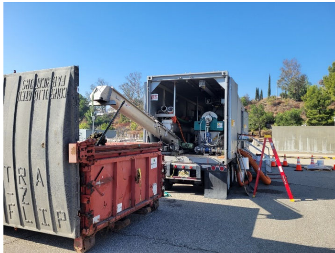
Staff dewatering centrifuge demonstration unit at Jensen plant
