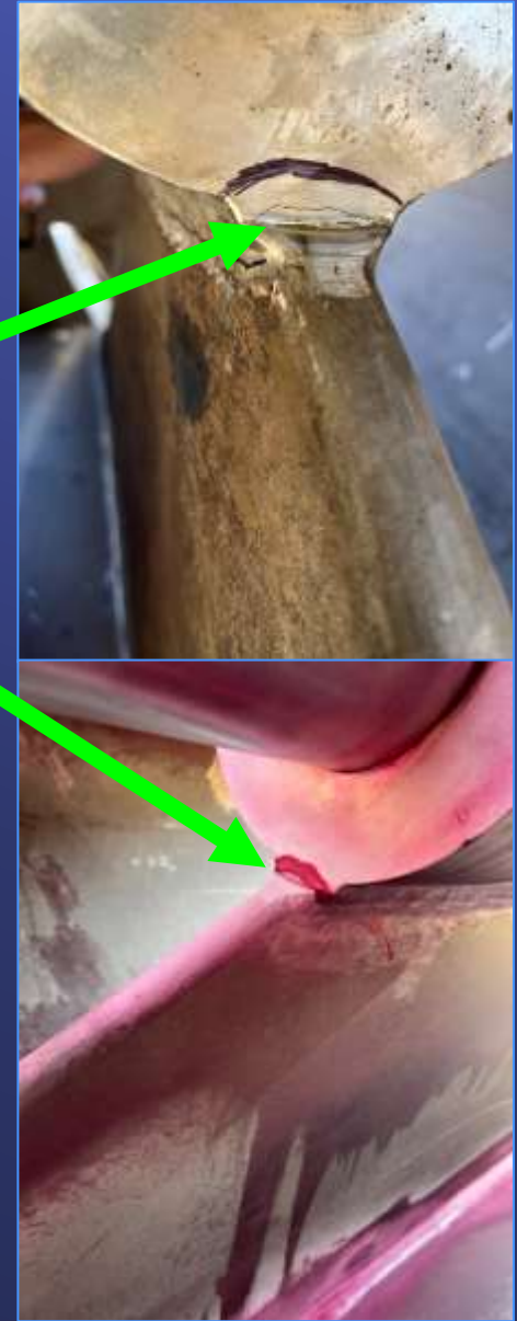
Liquid penetrant testing on valve body
