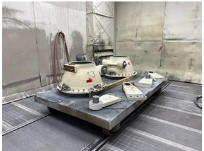
As-received valve bodies in blast booth
