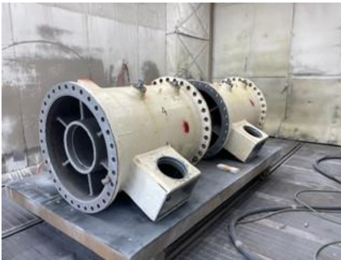
As-received valve bodies in blast booth
