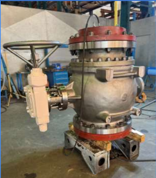
New 20" triple offset ball valve
