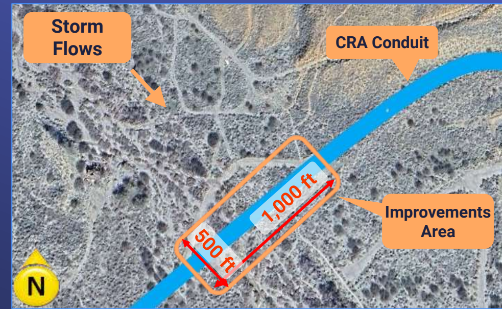
Erosion Control Improvements Area
