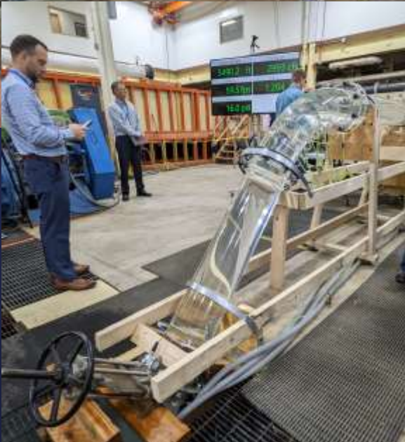
1/32 nd Scale Outlet Works Cavitation Model
