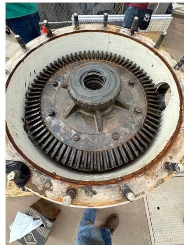
Damaged gate shaft (left and center) and as-found actuator assembly (right) for the gate at Copper Basin
