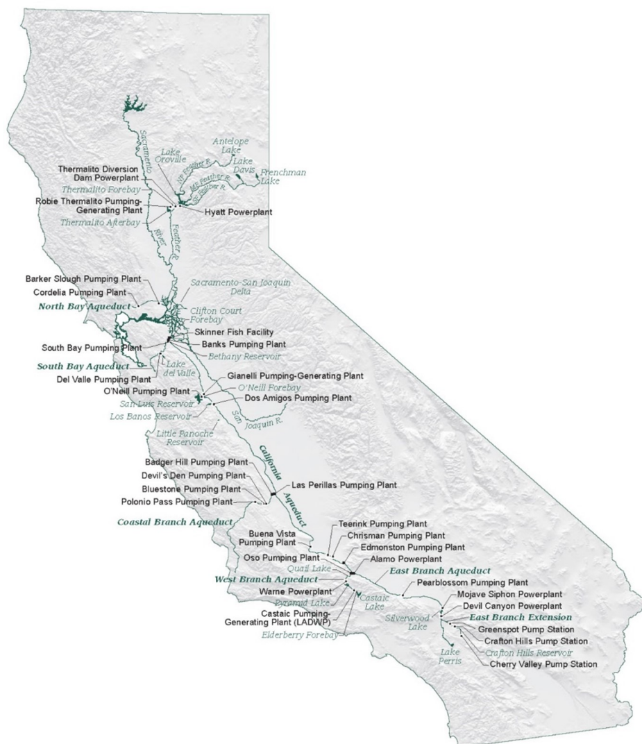
Figure 4: Facilities of the State Water Project
