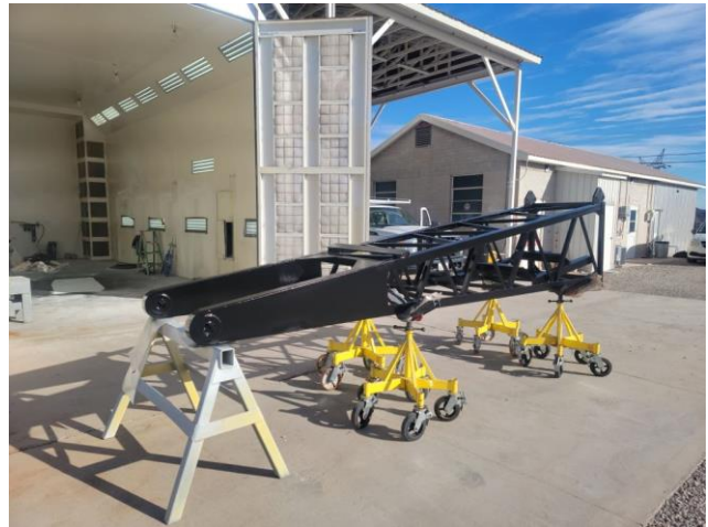
Refurbishment of a 20-foot jibboom for a mobile crane at a desert facility
