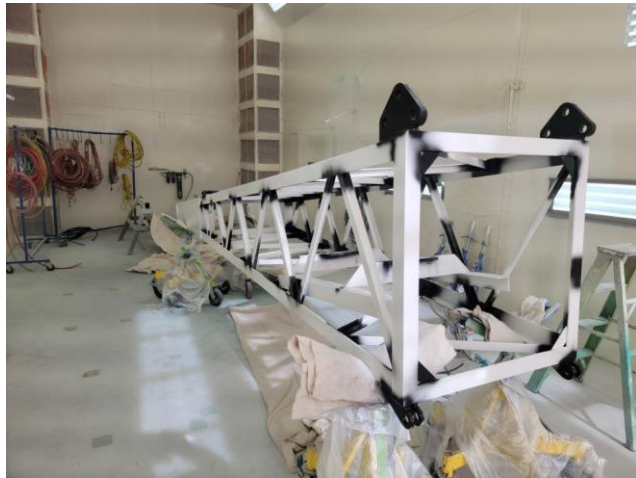
Refurbishment of a 20-foot jibboom for a mobile crane at a desert facility
