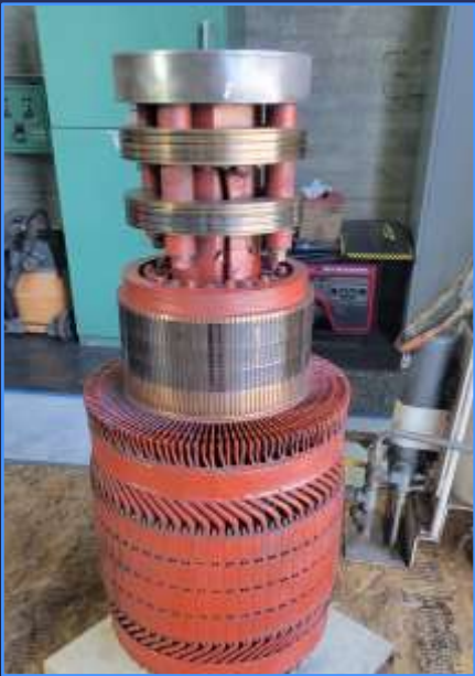
Brush Type Motor Exciter (Typ.)
