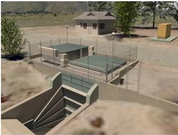
Digital design file of new Cabazon Wasteway Radial Gate and roof structure.
