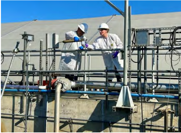
Staff collects water samples to assess bioreactor microbial concentrations at the demonstration plant
