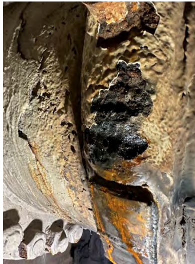
Close-up of the venturi meter leaking because of corrosion at the Santa Monica Feeder
