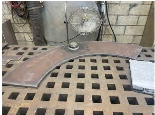
Fitting components for the repair of the Palos Verdes Feeder in various stages of fabrication
