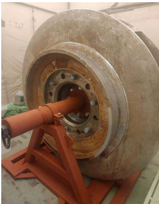
Main pump impeller cleaning and repair at Eagle Mountain pumping plant
