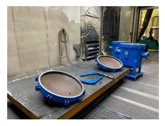
As-received set of quagga filters received (left) and prepping for abrasive blast of filters (right)
