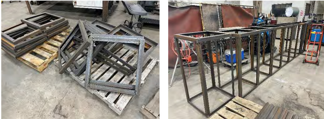
Fabrication of the cage tops (left) and cage structures (right)
