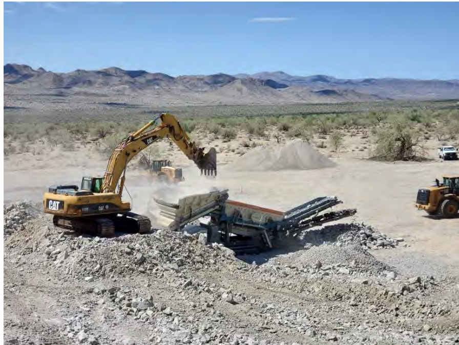
Staff operating a portable screening plant for aggregate material to maintain CRA access roads
