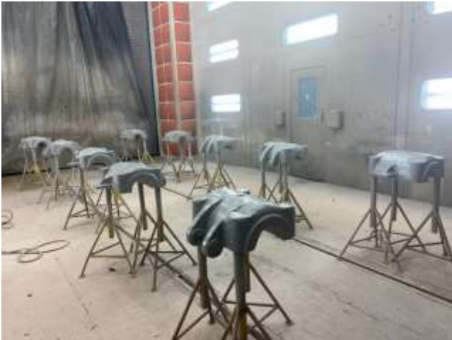
Finished coating of couplings (left) and palletized refurbished couplings (right) for DWR's San Luis Dam Head Gate
