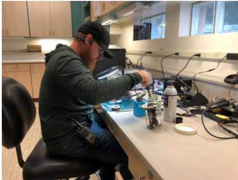
Staff replacing faulty microchips on a flow meter used to dose water treatment chemicals at the Skinner plant
