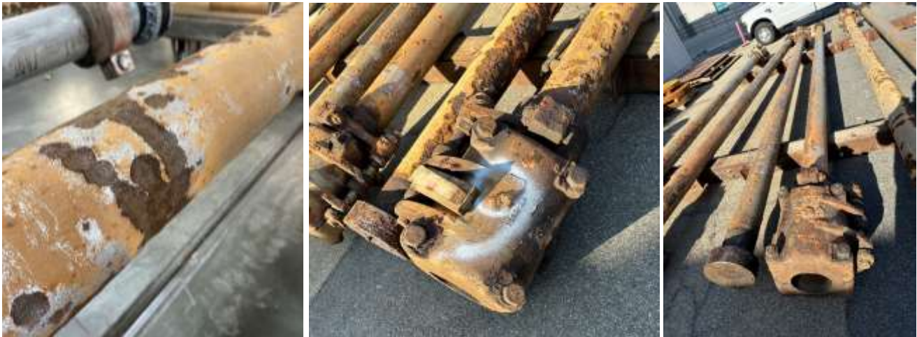
As-received stems (left), couplings (center), and clamps (right) for DWR's San Luis Dam Head Gate
