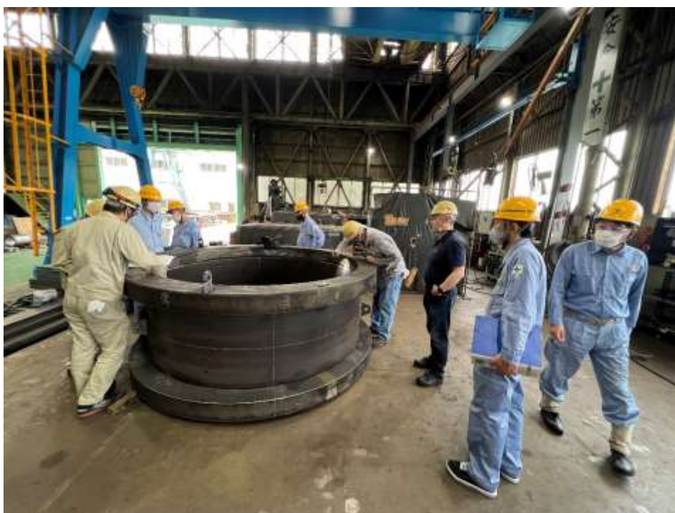
Badlands Tunnel Surge Tank Project —Valve inspection by Metropolitan staff and contractor personnel
