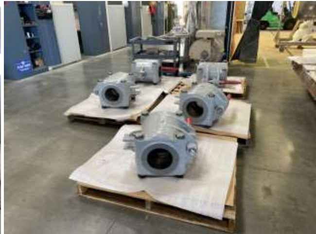
Finished coating of couplings (left) and palletized refurbished couplings (right) for DWR's San Luis Dam Head Gate
