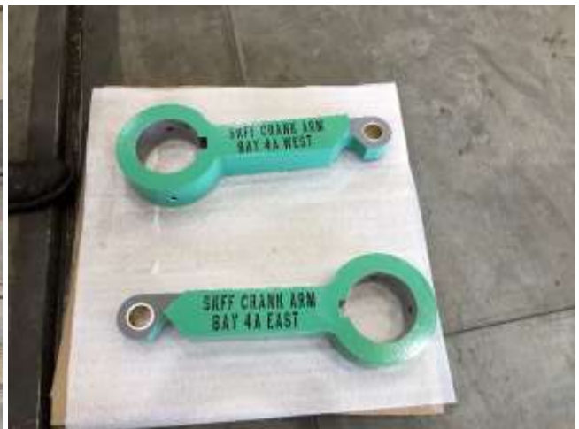
Finished coating of pillow blocks and drive shafts (left) and stenciling of finished crank arms (right) for DWR
