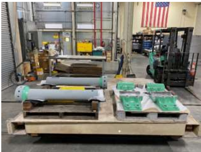
Finished coating of pillow blocks and drive shafts (left) and stenciling of finished crank arms (right) for DWR
