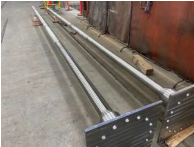
Completed manufacturing of center post (left) and machining of the gate's lower bearing (right) for DWR
