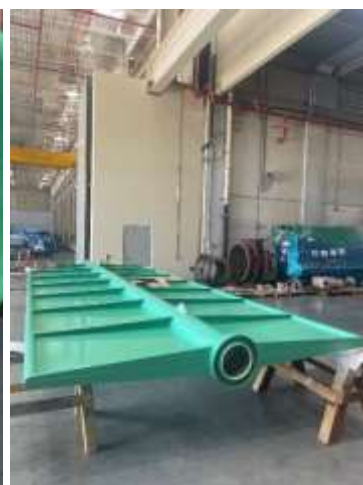
Test fit of internal components (left) and completed gate with finished coating (right) for DWR
