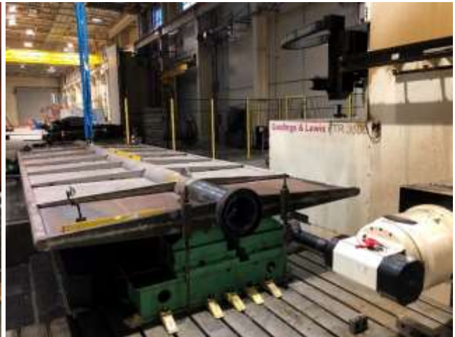
Completed manufacturing of center post (left) and machining of the gate's lower bearing (right) for DWR
