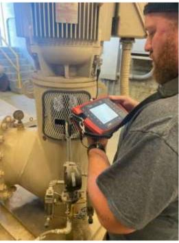
Staff performing vibration testing on a used washwater return pump at the Diemer plant
