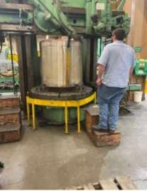
Staff weld-repairing valve gate (left) and machining of inner valve body (right) for Red Mountain PCS
