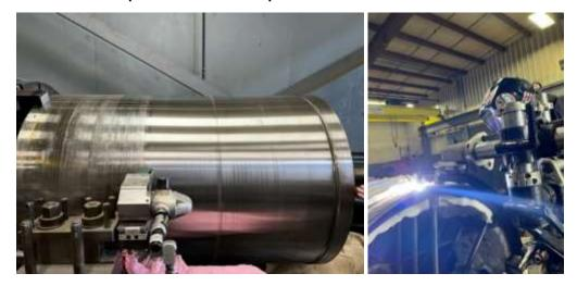
Vendor performing machining work (left) and overlaying hard-face material on valve gate (right) for Red Mountain PCS
