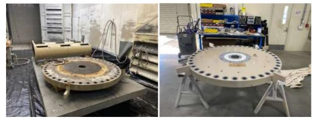
As-found sleeve valve cover (left) and completed valve cover (right) for Red Mountain PCS
