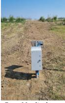
Sensoil - Upper Levee Zone Monitoring
