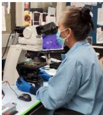
Staff examining water samples for quagga mussel veligers by cross-polarized microscopy
