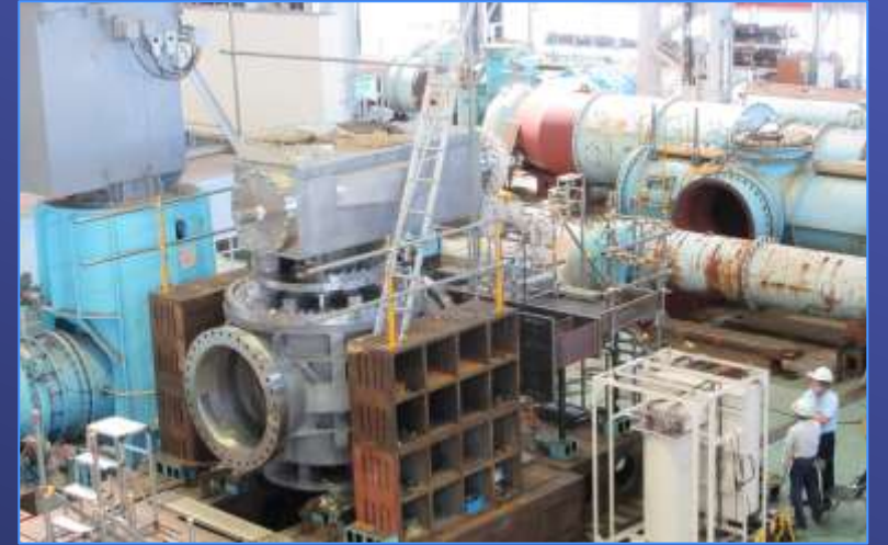
Fabrication of 48-inch Diameter Valve
