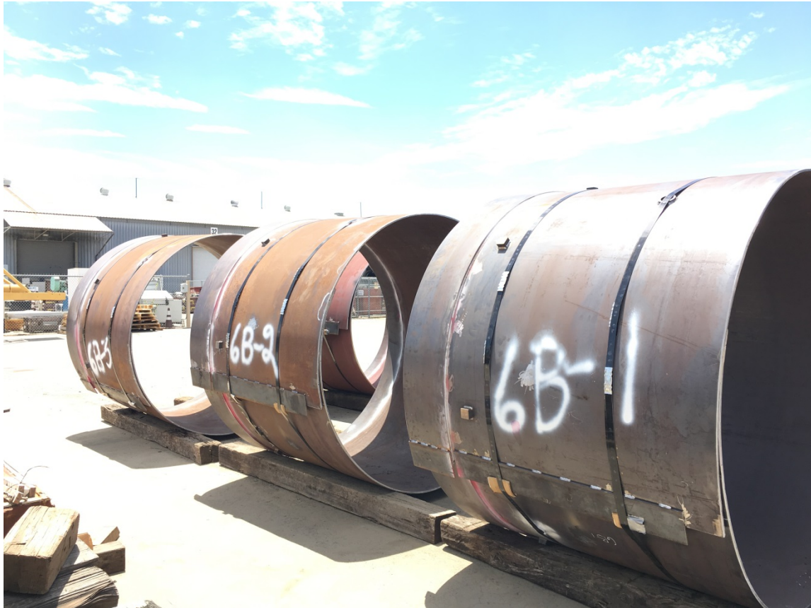
Figure 3-3. Collapsed Steel Pipe Section
