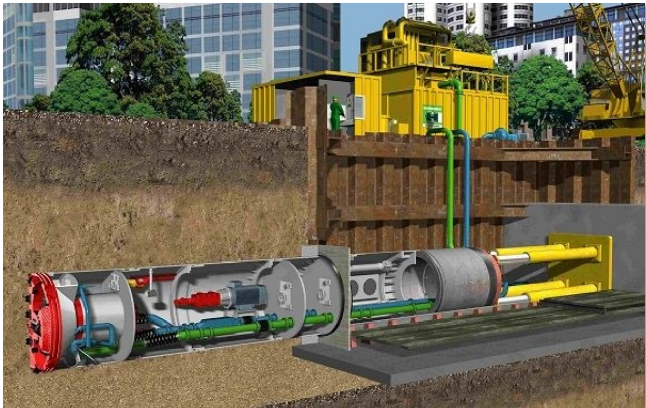
Example of micro-tunneling technology that will be used for the Perris Valley Pipeline – Tunnels project
