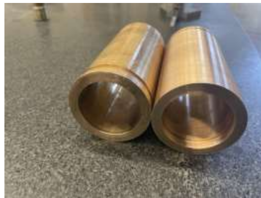
New bronze bushings manufactured to replace the worn stainless-steel bushings for Perris Pumpback facility
