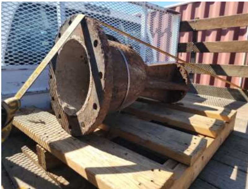
Before (left) and after (right) blasting and coating of circulating water pump components for Eagle Mountain pumping plant
