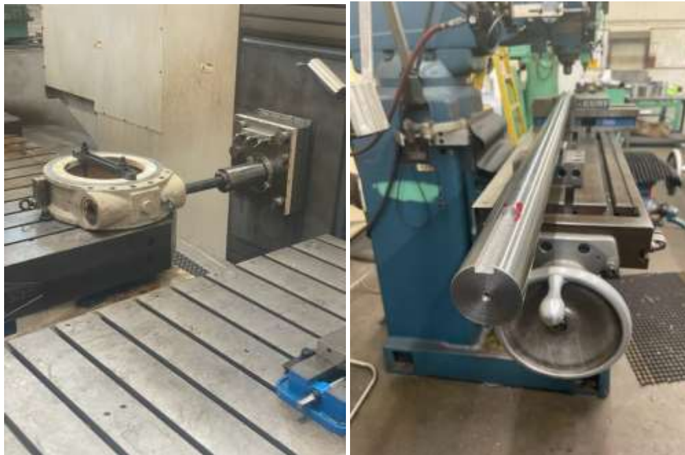
Removal of compromised stainless-steel bushing from valve body (left) and machining of new shaft (right) for Perris Pumpback facility
