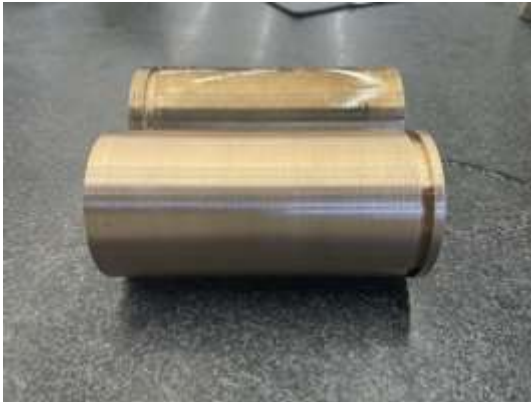
New bronze bushings manufactured to replace the worn stainless-steel bushings for Perris Pumpback facility
