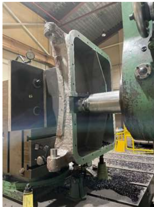
Staff machining a scroll case door to remove a corroded flange for DWR's Gianelli facility
