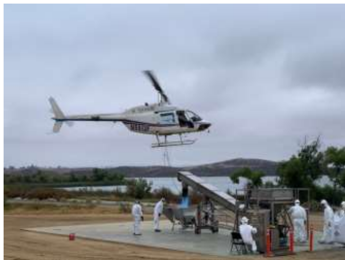
Staff loading copper sulfate into the hopper/spreader for application at Lake Skinner
