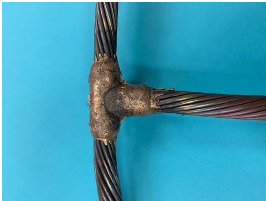
Finished connection using exothermic welding
