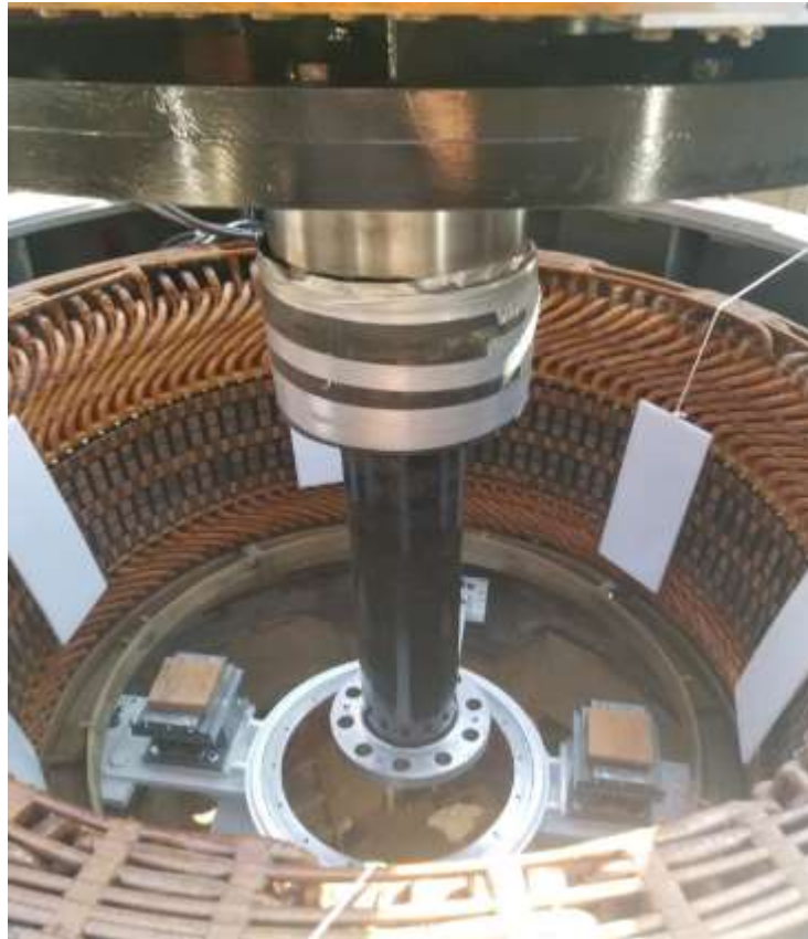
Red Mountain HEP reconditioned generator rotor and stator
