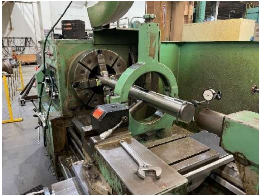
Machining of stainless-steel shafts for Red Mountain PCS at the La Verne Shops
