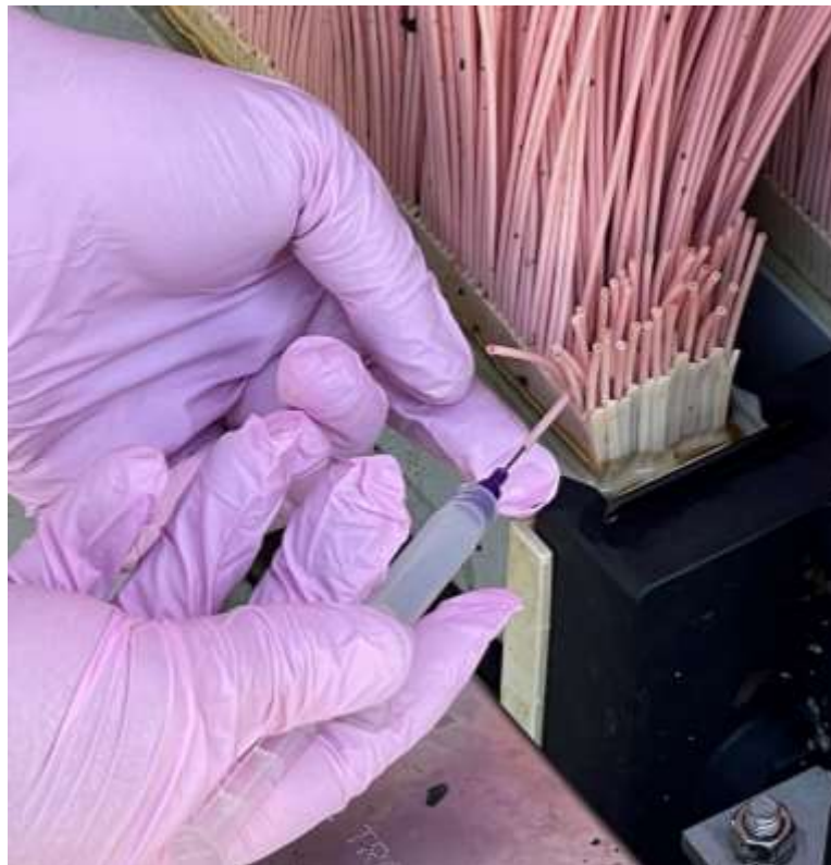
Staff seal cut fibers in the MBR to restore membrane integrity before challenge testing
