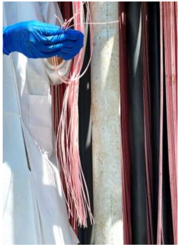
Staff cut and inspect fibers from the MBR to restart a challenge test at the demonstration facility
