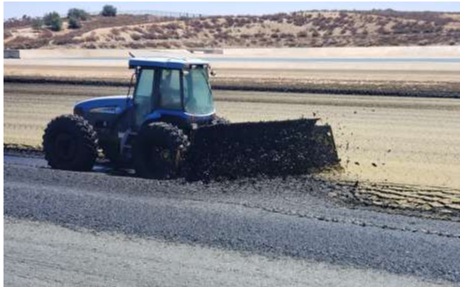
Brown Bear agitating wet solids at the Mills plant
