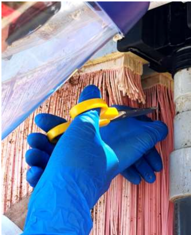
Staff cut and inspect fibers from the MBR to restart a challenge test at the demonstration facility
