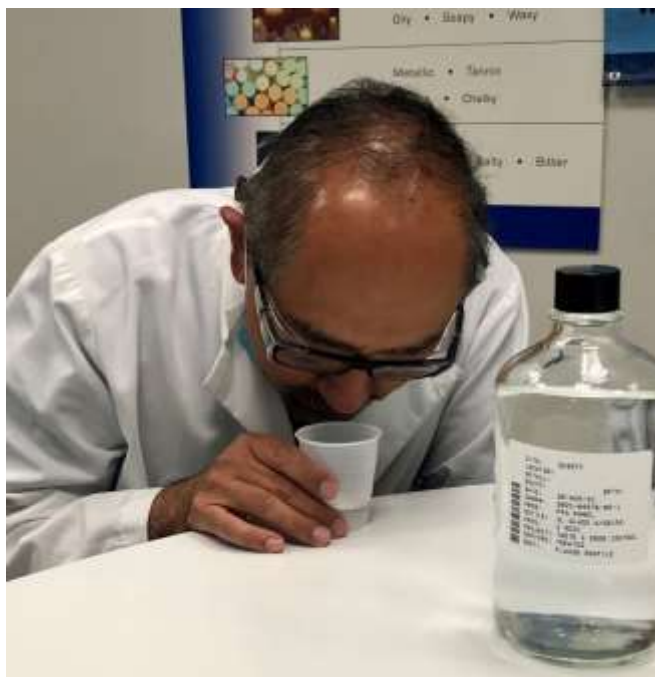
Staff conducting Flavor Profile Analysis of water sample to resolve odor event
