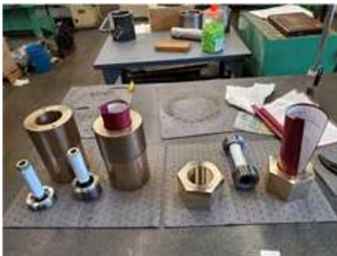
Manufactured lift and capture nuts for Red Mountain PCS
