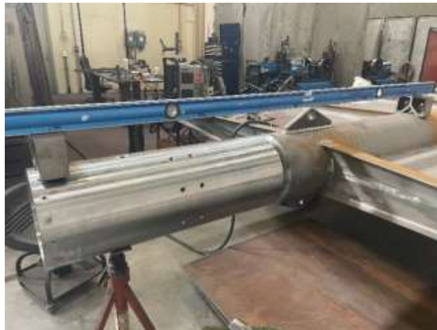
Replacement of gate section (left) and new center post (right) for DWR's Banks Pumping Plant
