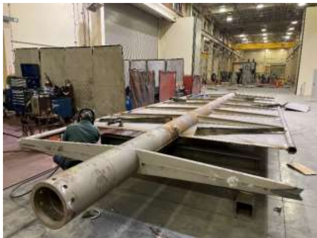
Replacement of gate section (left) and new center post (right) for DWR's Banks Pumping Plant
