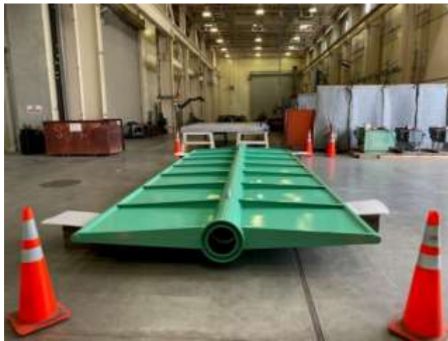
DWR's wing gate before (left) and after (right) refurbishment at the La Verne Shops
