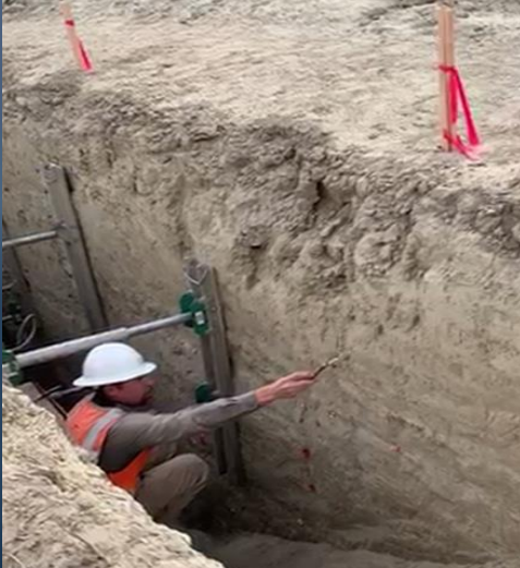
Fault Trenching Study
