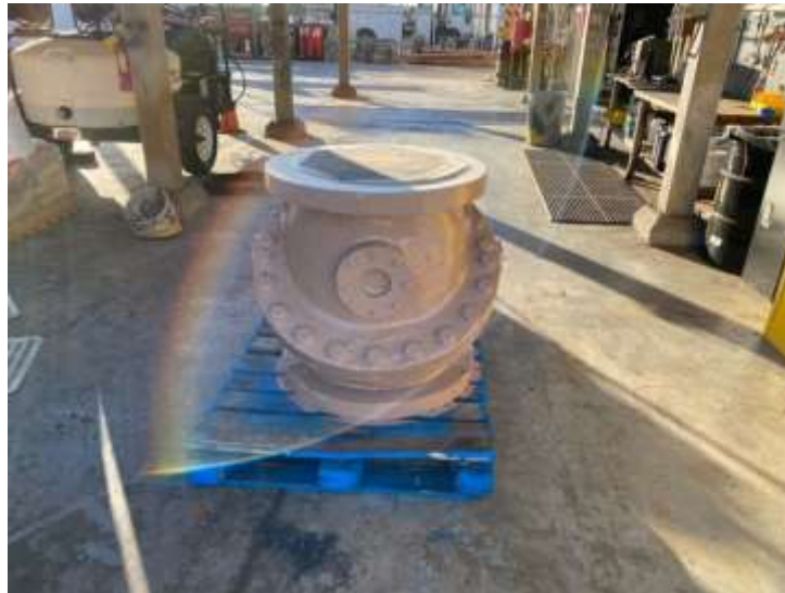
Finished 300 lb. slanted disc check valve ready to be shipped to the Greg Avenue pump station
