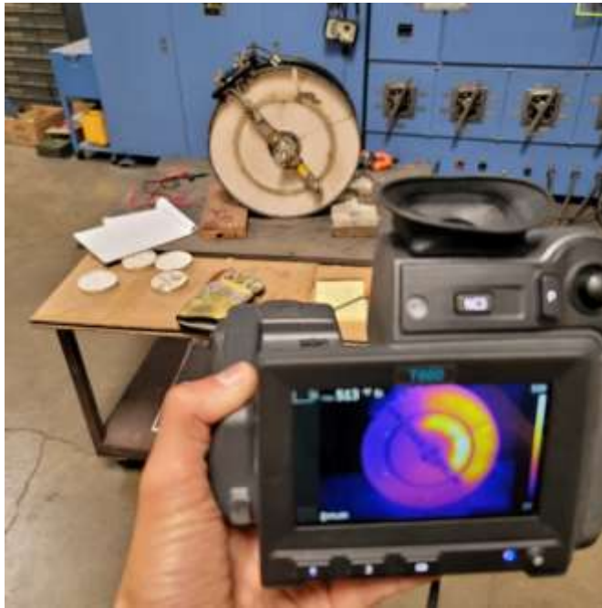
Staff taking temperature readings during testing (left) and new insulation material filled (right) for the rheostat at Eagle Mountain pumping plant
