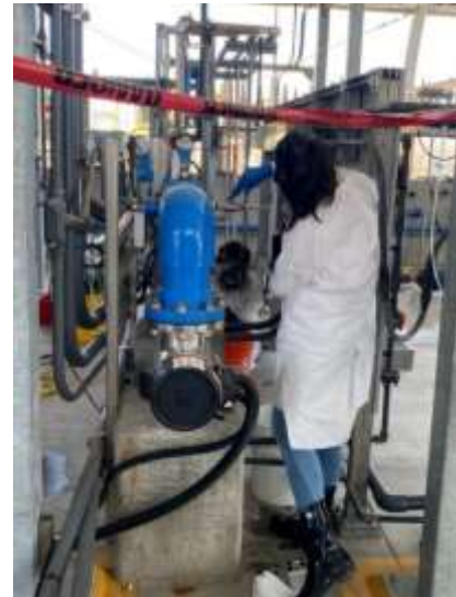
Consultant staff perform 1,4-dioxane challenge testing on the advanced oxidation process at the demonstration facility
