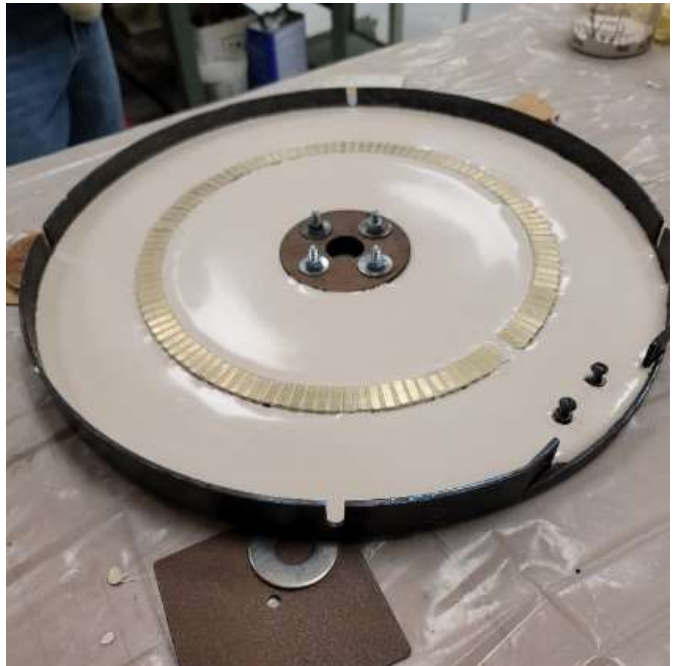
Staff taking temperature readings during testing (left) and new insulation material filled (right) for the rheostat at Eagle Mountain pumping plant
