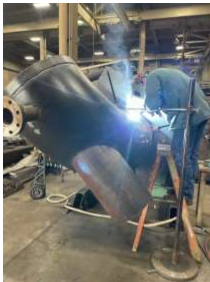
La Verne Shops staff fabricating a surge tank connection for the Greg Avenue pump station
