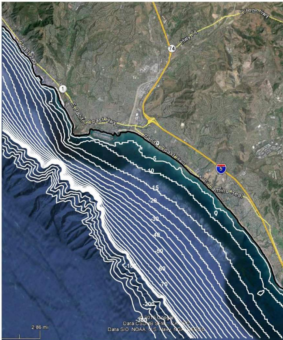
Figure 6.2: Near-field refraction/diffraction grid to simulate shoaling waves in the immediate neighborhood of Dana Point, SJCOO and Doheny Beach.
