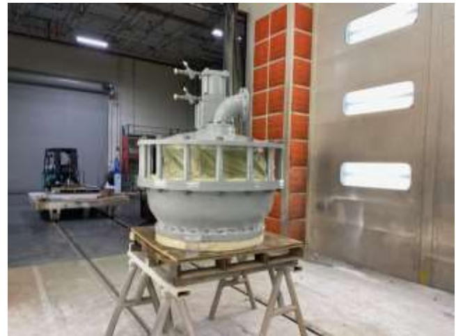
Surface preparation of siphon breaker for coating (left) and curing of applied coating (right) for DWR's Dos Amigos Pumping Plant
