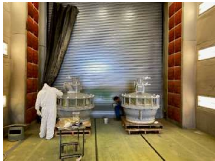
Fully assembled & tested siphon breakers (left) and application of finished coating (right) for DWR's Dos Amigos Pumping Plant
