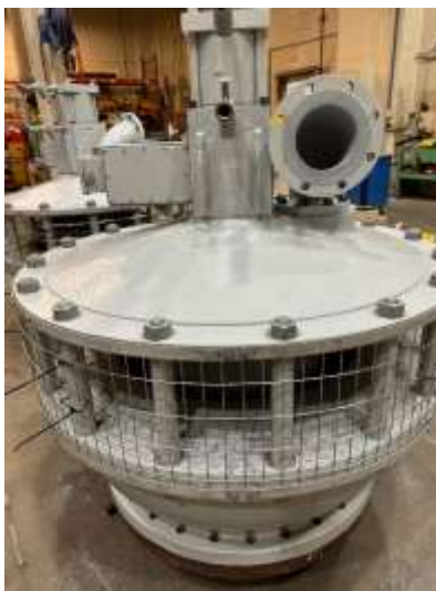
Fully assembled & tested siphon breakers (left) and application of finished coating (right) for DWR's Dos Amigos Pumping Plant
