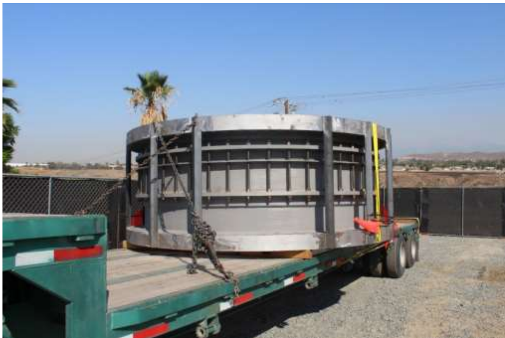
The La Verne Shops manufactured a new slip joint for the Upper Feeder leak repair
