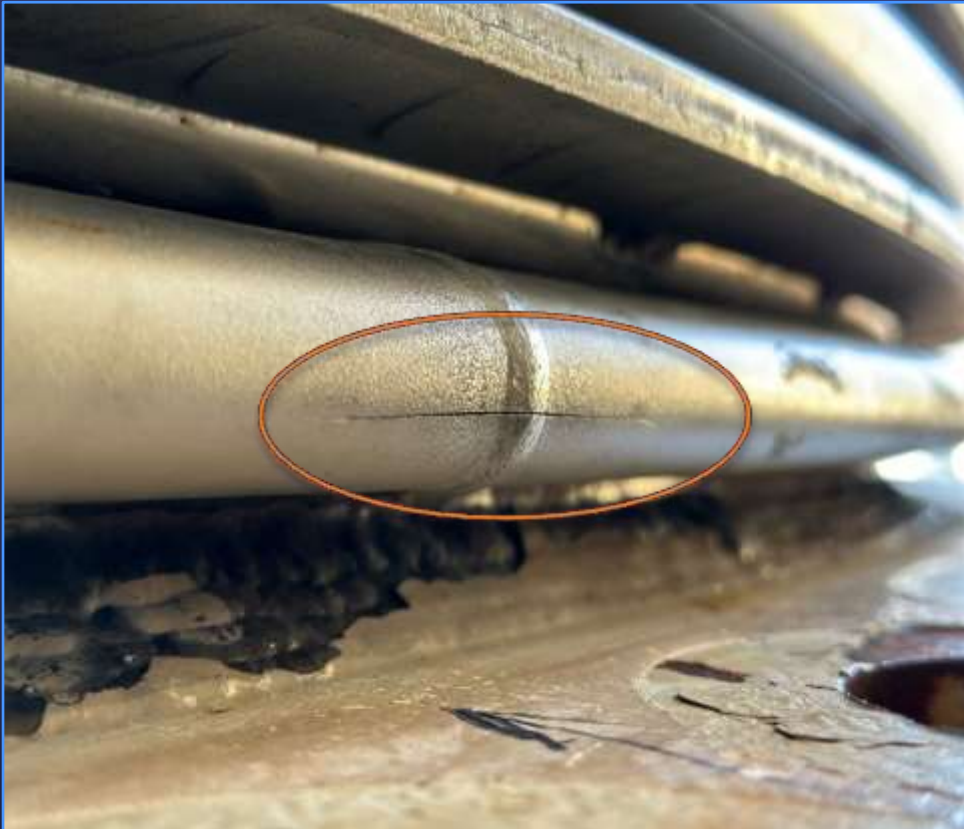
Bellows joint 2.5-inch crack
