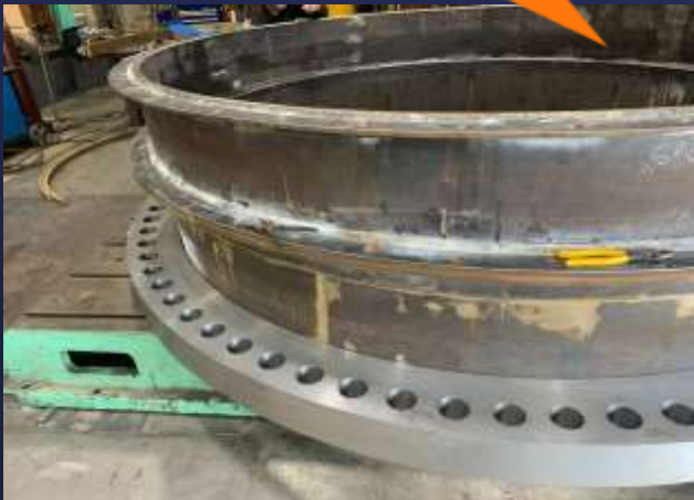
New Slip Joint Fabrication @ La Verne Shops
