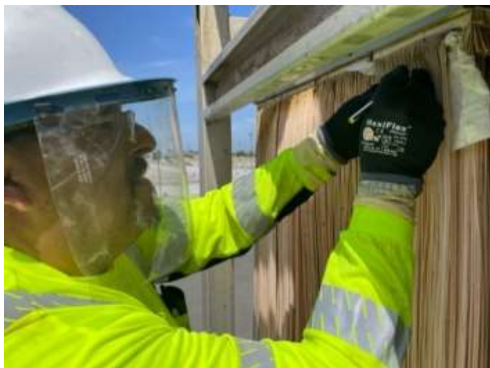
Staff intentionally damaging MBR fibers for challenge testing (left) and reinstalling the MBR cassette (right) at the demonstration facility
