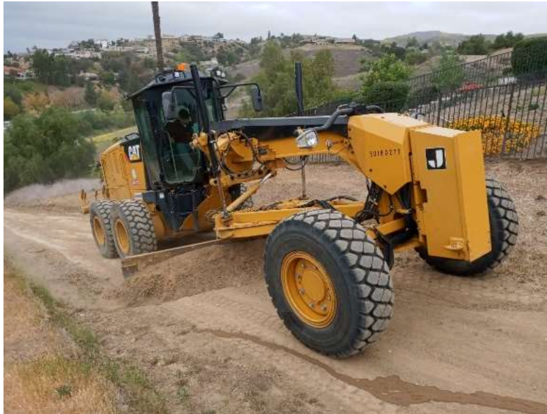
Staff using a motor grader for patrol road repairs along the Lower Feeder
