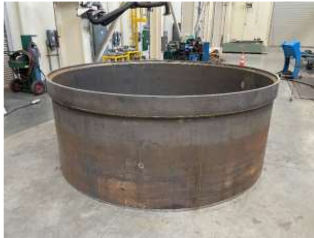
Fabrication of new 113-inch slip joint to replace leaky bellows joint on Upper Feeder
