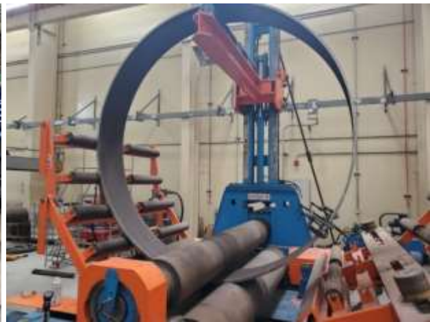
Fabrication of new 36-inch accessway (left) and rolling of new slip joint ring (right) to facilitate leak repairs on the Upper Feeder
