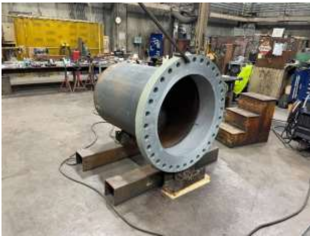
Fabrication of new 36-inch accessway (left) and rolling of new slip joint ring (right) to facilitate leak repairs on the Upper Feeder
