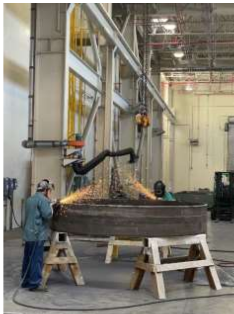
Staff welding new slip joint ring for Upper Feeder repairs
