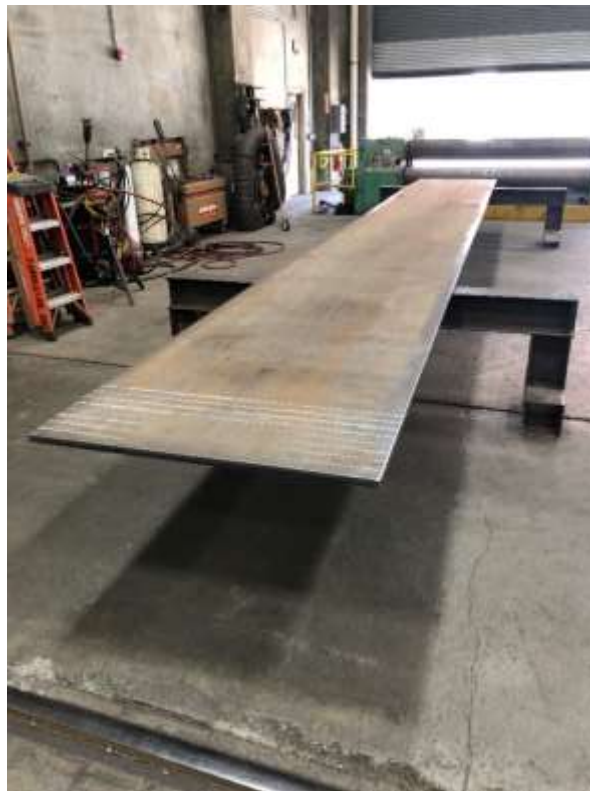
Rolling of new carbon steel slip joint in the La Verne Shops for Upper Feeder repairs
