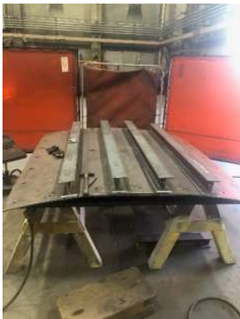
Bulkhead fabrication (left) and installation by divers (right) at the Lake Skinner outlet tower
