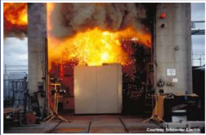
Switchgear undergoing arc flash testing (Stock image – Not a Metropolitan facility)
