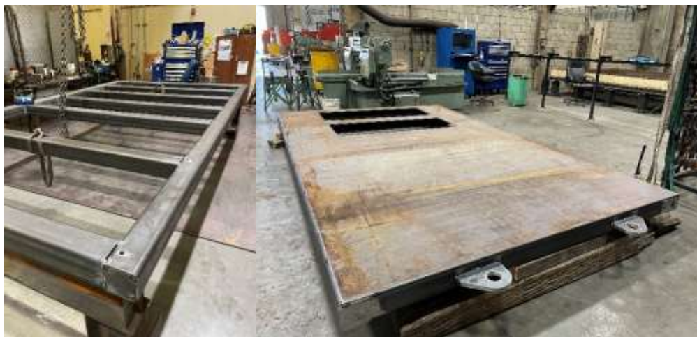
Fabrication of gate frame (left) and installed gate skin with square openings (right) for Desert pumping plants
