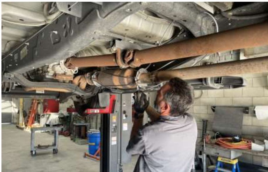
Metropolitan Fleet staff installing CatClamp theft deterrent device on Valley C&D utility vehicle
