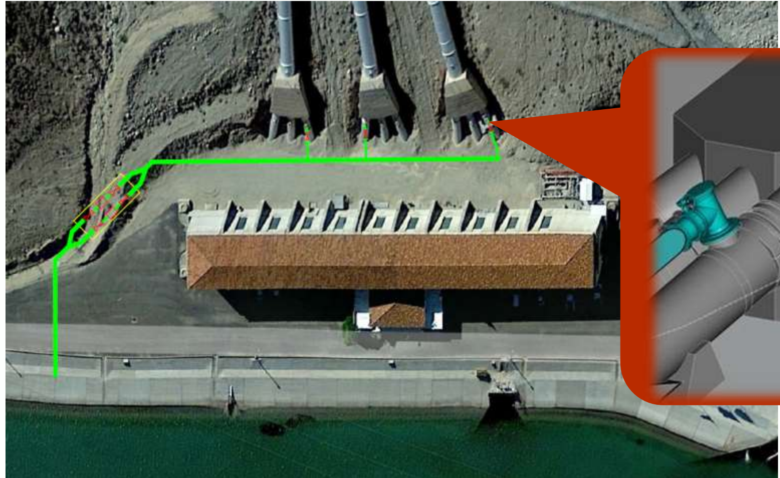
Recirculation line connections at the Eagle Mountain Pumping Plant
