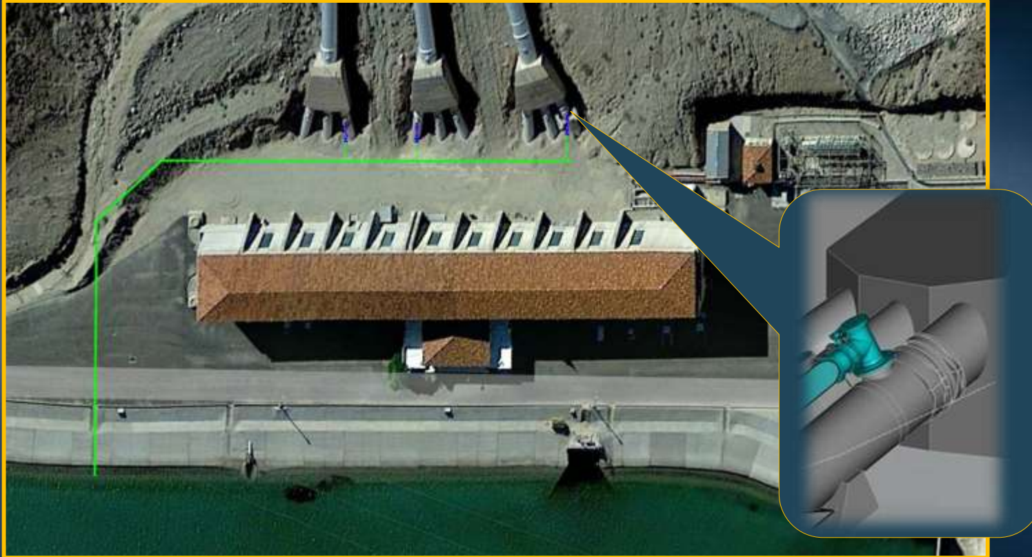
Recirculation Line Connections at the Eagle Mountain Pumping Plant
