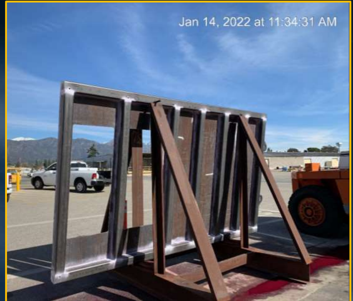
Orifice Gate in fabrication for Iron Mtn Pumping Plant
