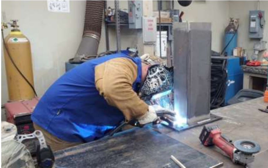
Staff welding a new pedestal for Module 7 traveling bridge electrical cable reel at the Skinner plant
