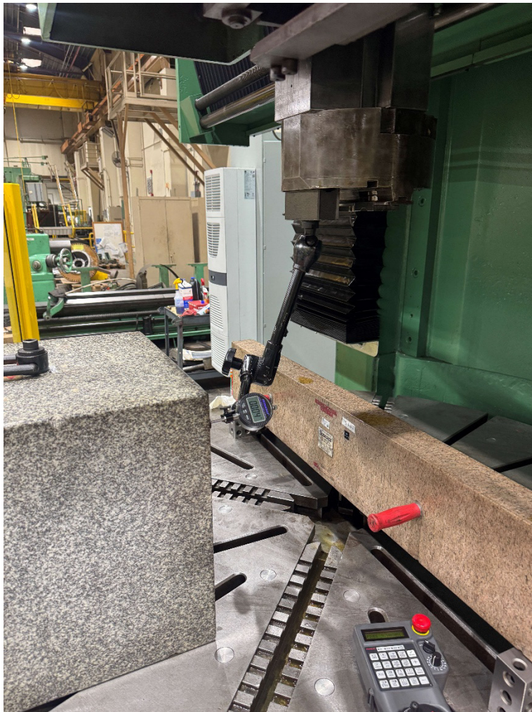
La Verne Shops Improvements – Testing Refurbished Vertical Turning Lathe
