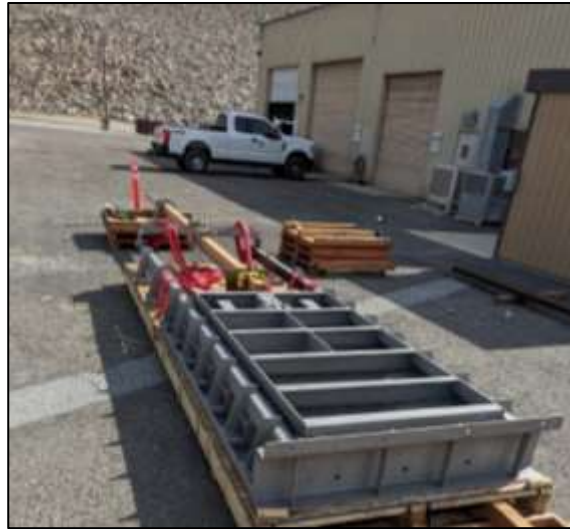
The new replacement gate for Lake Mathews Forebay
